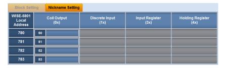
• After all Coil Output settings of the Modbus RTU Slave module are completed, click "Save" button to save the changes.
