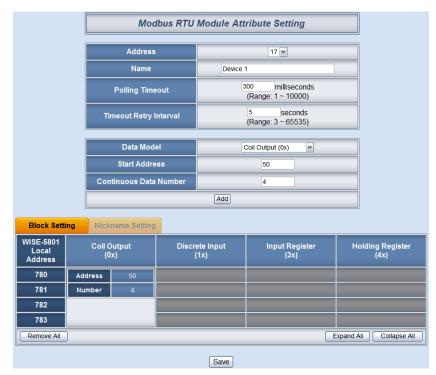
Figure 4-24: Modbus RTU Slave Module Coil Output Setting Example
