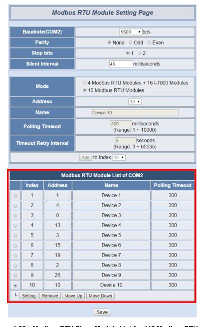
Figure 4-22: Modbus RTU Slave Module List for "10 Modbus RTU Modules"
