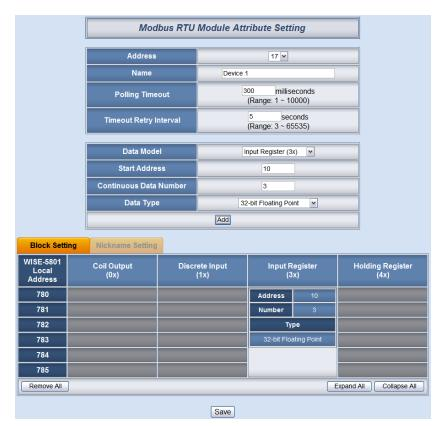
Figure 4-28: Modbus RTU Slave Module Input Register Setting Example
