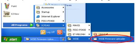
Figure 10-9: Launch WISE Firmware Uploader
