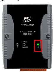
4. Power off WISE-580x and switch Rotary Switch back to "0" position. Power on WISE-580x again, the WISE-580x will be restored to factory default settings.
