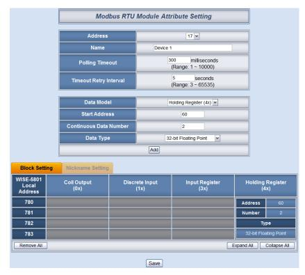
Figure 4-30: Modbus RTU Slave Module Holding Register Setting Example
