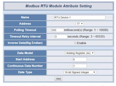
Figure 4-29: Modbus RTU Slave Module Holding Register Setting Page
