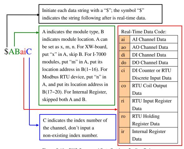
Figure 5-16: SMS Command Data Retrieve Coding Rules
