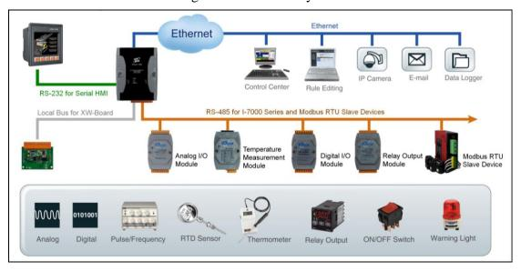
Figure 1-1: WISE-580x System Architecture
