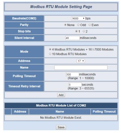
Figure 4-20: Modbus RTU Slave Module Setting Page
