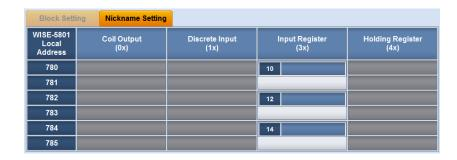
• After all Input Register settings of the Modbus RTU Slave module are completed, click "Save" button to save the changes.
