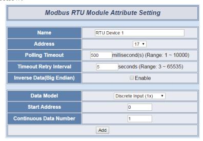
Figure 4-25: Modbus RTU Slave Module Discrete Input Setting Page
