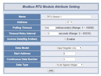
Figure 4-27: Modbus RTU Slave Module Input Register Setting Page
