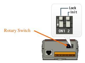
2. Switch Rotary Switch to position 1 to restore to factory default, the position of Rotary Switch indicates:
