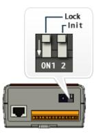
Figure 2-1: The Init Switch on the controller
