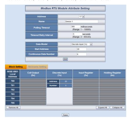
Figure 4-26: Modbus RTU Slave Module Discrete Input Setting Example
