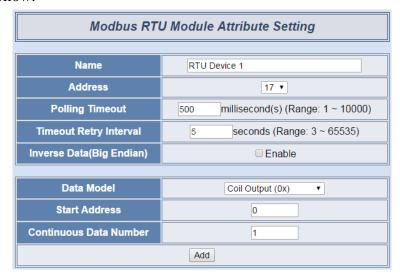
Figure 4-23: Modbus RTU Slave Module Coil Output Setting Page
